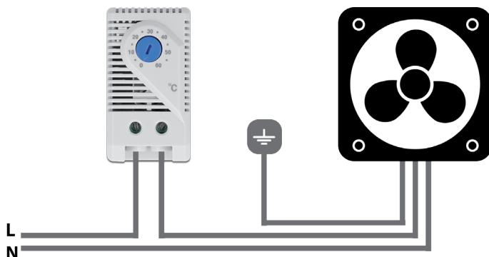
Normally open contact (switching contact closes when temperature rises)
