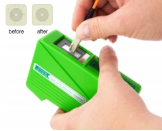
cleaning of fiber optic connectors
